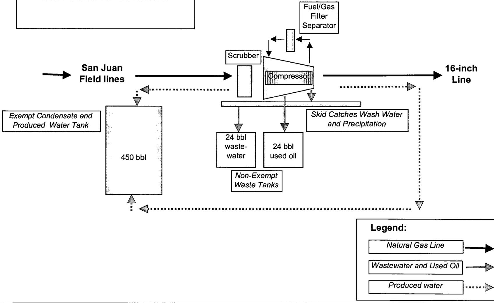
Plate 1: Process Map of the Hart #3 Compressor Station
