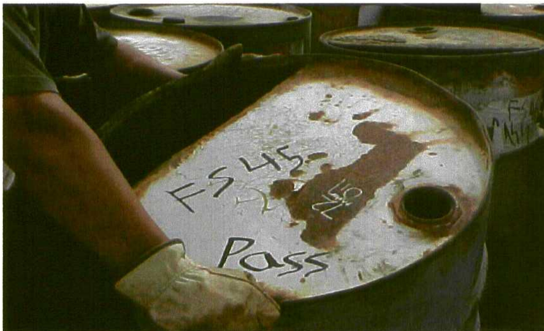
Photo 1: Photograph showing the labeling used during the transfer process. The pass/fail labels identify the drums as containing chlorinated solvents in excess of 1000 ppm or not.
