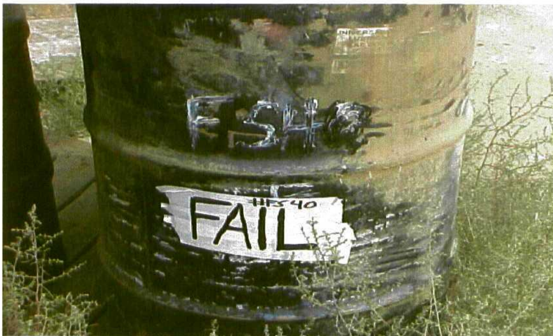
Photo 2: Photograph showing the labeling used during the transfer process. The pass/fail labels identify the drums as containing chlorinated solvents in excess of 1000 ppm or not.
