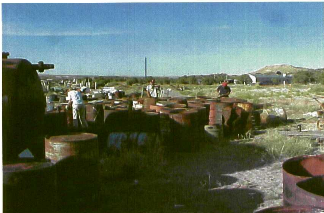
Photo 3: Photograph taken during the process of de-heading and crushing 55-gallon drums.
