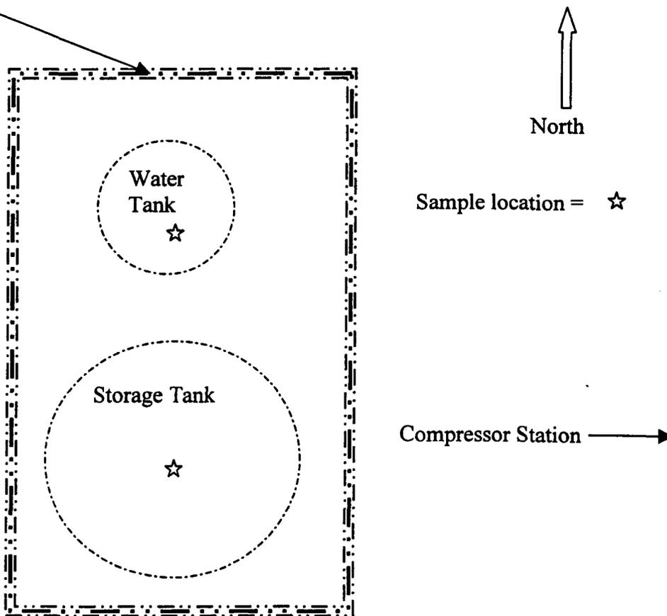
Sample from Water Tank collected at 8 feet PID field reading 0.0 ppm
