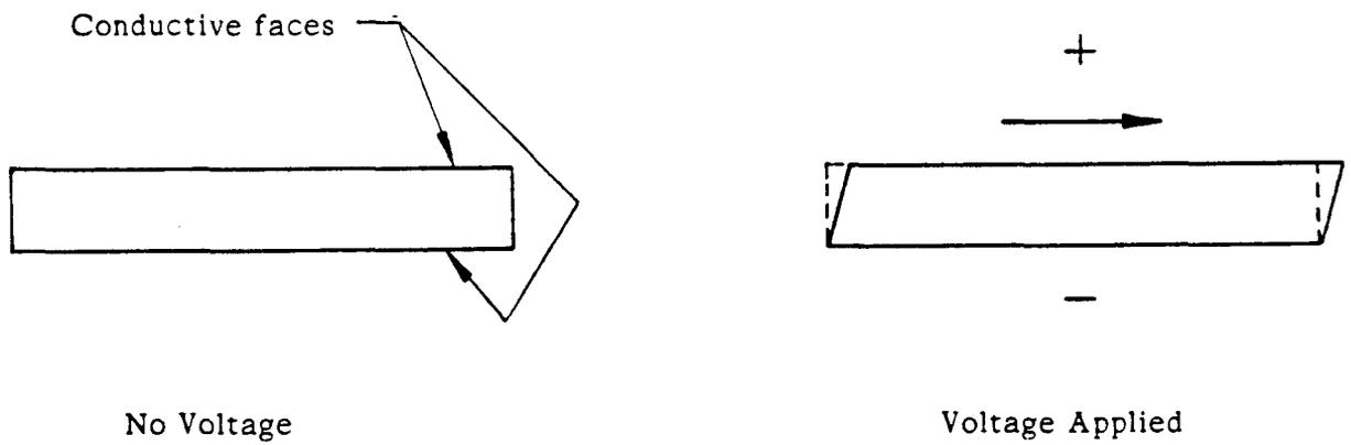
Figure 1. Shear and compressional transducer response to applied voltage.
