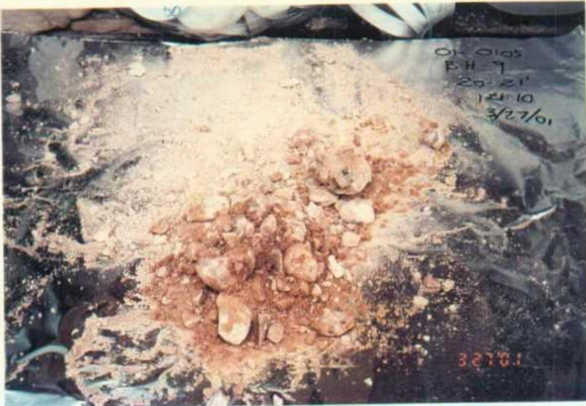
6. Soil Sample from Boring BH-9 (20 to 21 Feet BGS)
