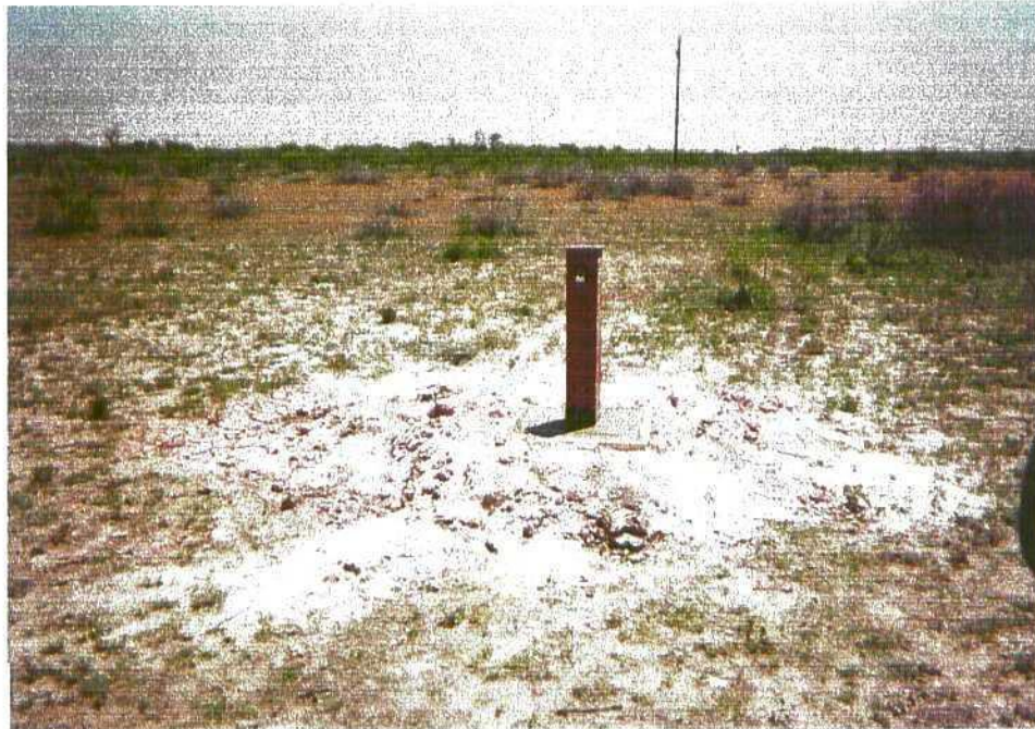
Photo 36: Completed monitor well MW-9.
