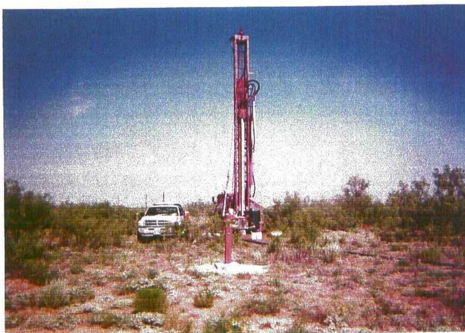
Photo 12: Drilling of soil boring S-13.
