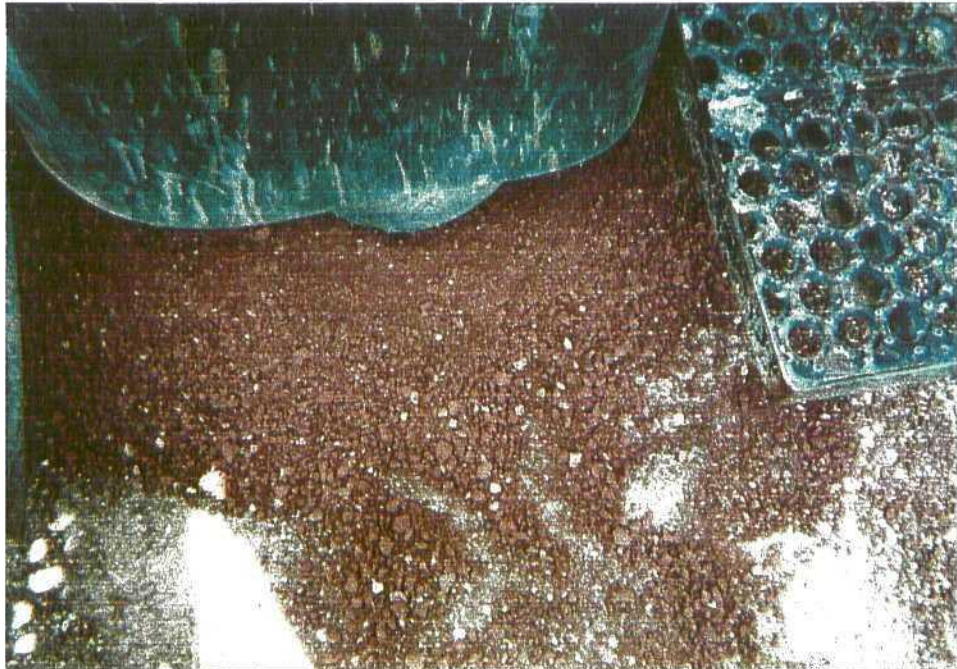
Photo 32: Underlying confining layer of the Ogallala Aquifer encountered in monitor well MW-8.
