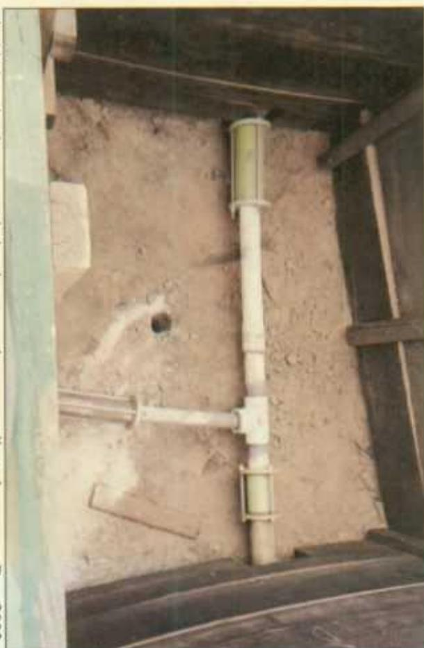
inside junction box; auger hole where samples were collected
