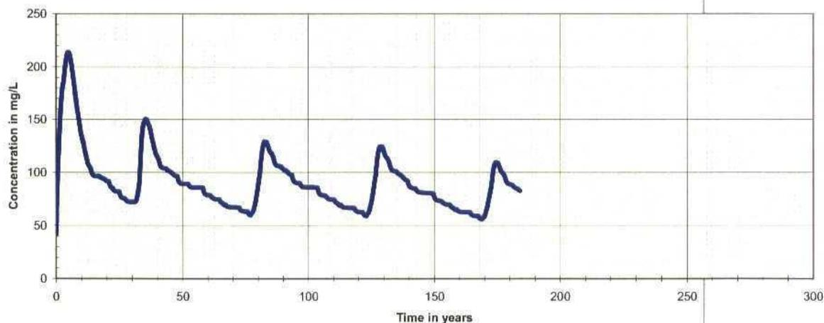
Figure 4b: Predicted Chloride Concentration in the Aquifer, BD-4 Site with Evapotranspiration Barrier Installed at Year 0 - Diamonds Represent Ground Water Samples in May and August 2006
