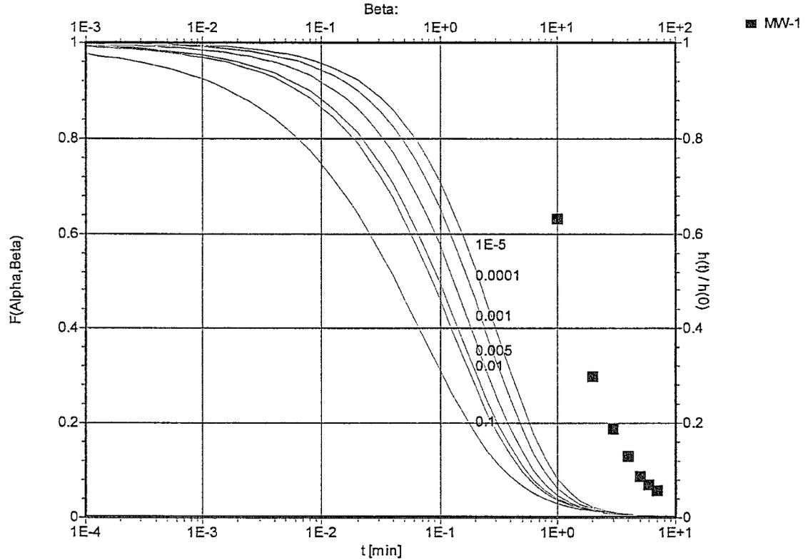
Slug Test: New Slug Test
