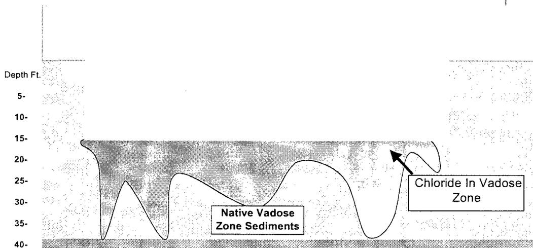
Note also that Figure 6 also assumes that the chloride concentration of the material from 5-13 is about 250 mg/kg, the same concentration as the average obtained from sampling the east spoil pile. From 0-5 feet, we assumed the background concentration of about 30 mg/kg.
