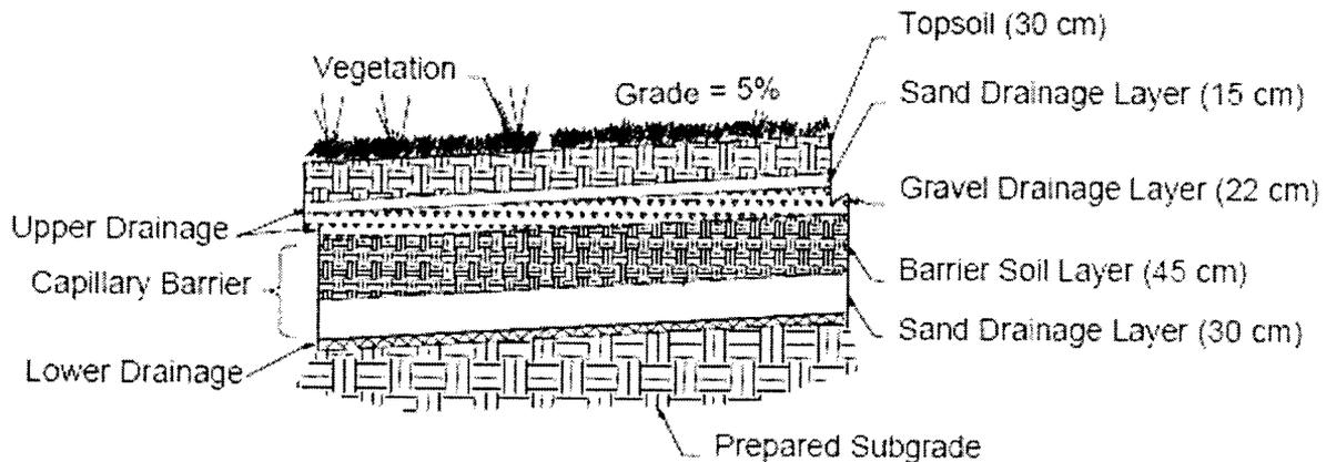
Profile of Alternative Test Cover 3 (Landfill 5)
