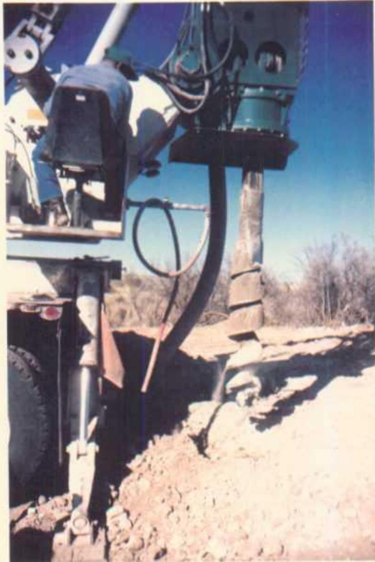
Photograph 5: Close-up of auger bit showing the generally dry nature of the subsurface materials.
