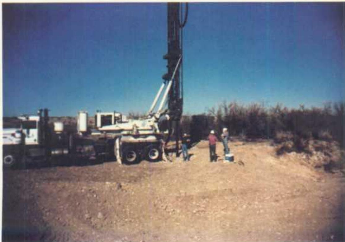
Photograph 2: Solid-stem auger drilling rig used to obtain soil samples.
