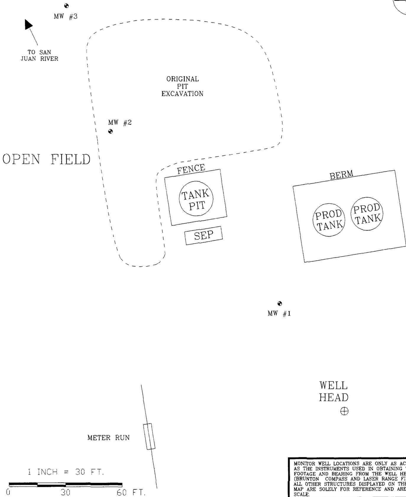
MONITOR WELL LOCATIONS ARE ONLY AS ACCURATE AS THE INSTRUMENTS USED IN OBTAINING THE FOOTAGE AND BEARING FROM THE WELL HEAD (BRUNTON COMPASS AND LASER RANGE FINDER). ALL OTHER STRUCTURES DISPLAYED ON THE SITE MAP ARE SOLELY FOR REFERENCE AND ARE NOT TO SCALE.
