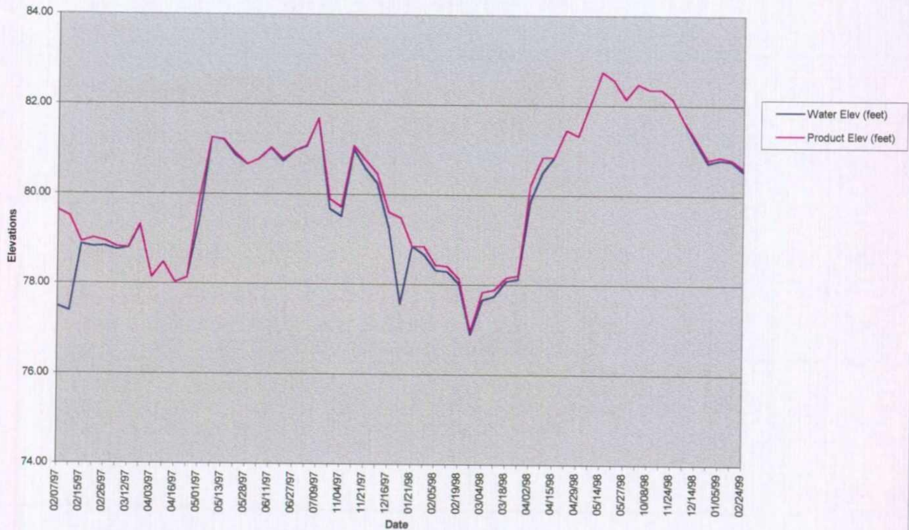
Water Level Elevations and Product Level Elevations vs. Time R-2
