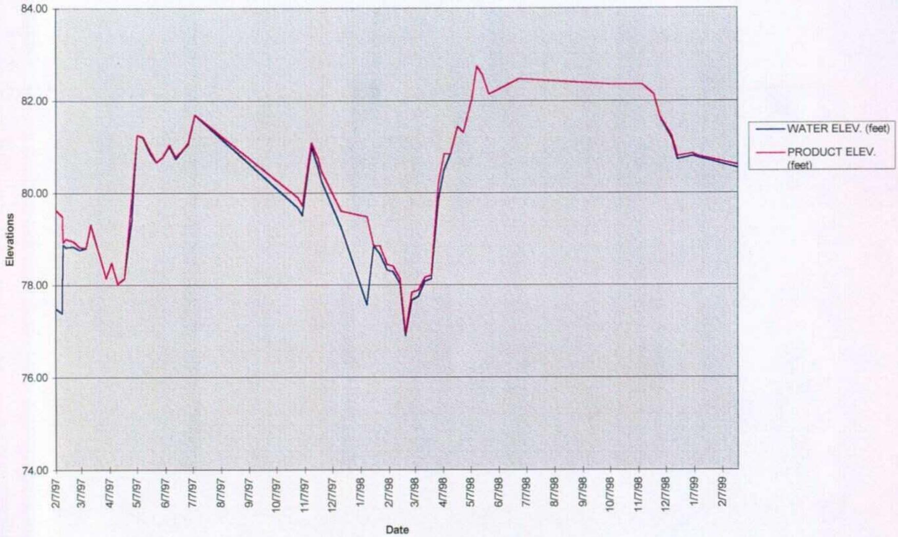
Water Level Elevations vs. Time
