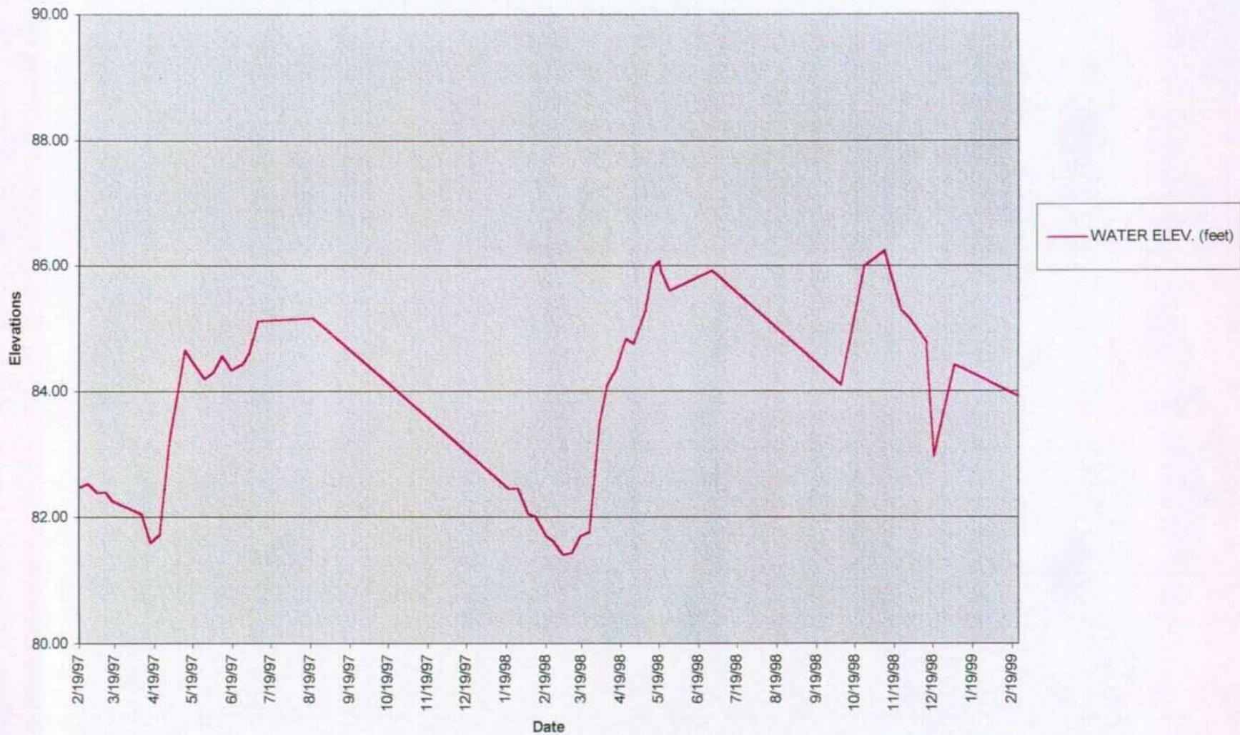
Water Level Elevation vs. Time
