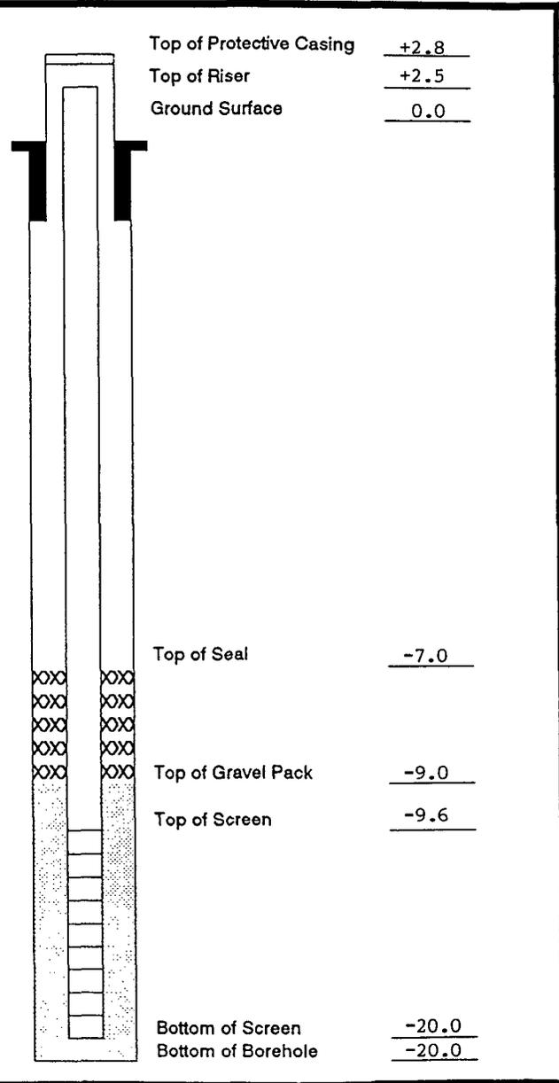
Comments: CLAY RING IN BOTTOM OF AUGERS WOULD NOT ALLOW PELLETS TO DROP THROUGH AUGERS. HAD TO PULL AUGERS TO SET SEAL. WATER LEVEL AT 12.25. NO PRODUCT (1630)
