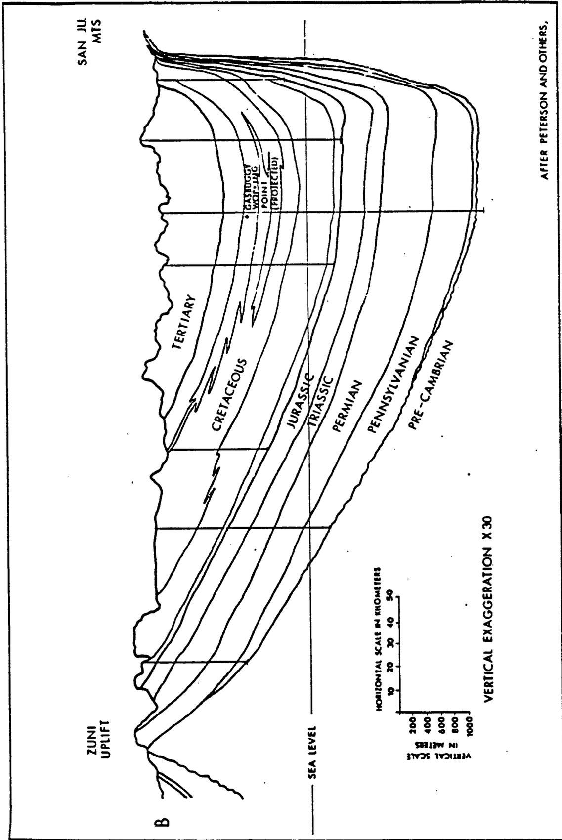
Figure 3. South-North Geologic Cross Section Across the San Juan Basin
