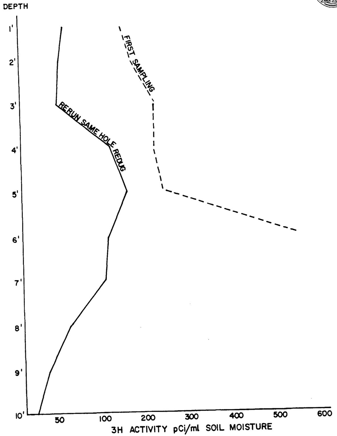
FIG. 6 TRITIUM ACTIVITY VS DEPTH FOR PROFILE HOLE 1 WI, Ø
