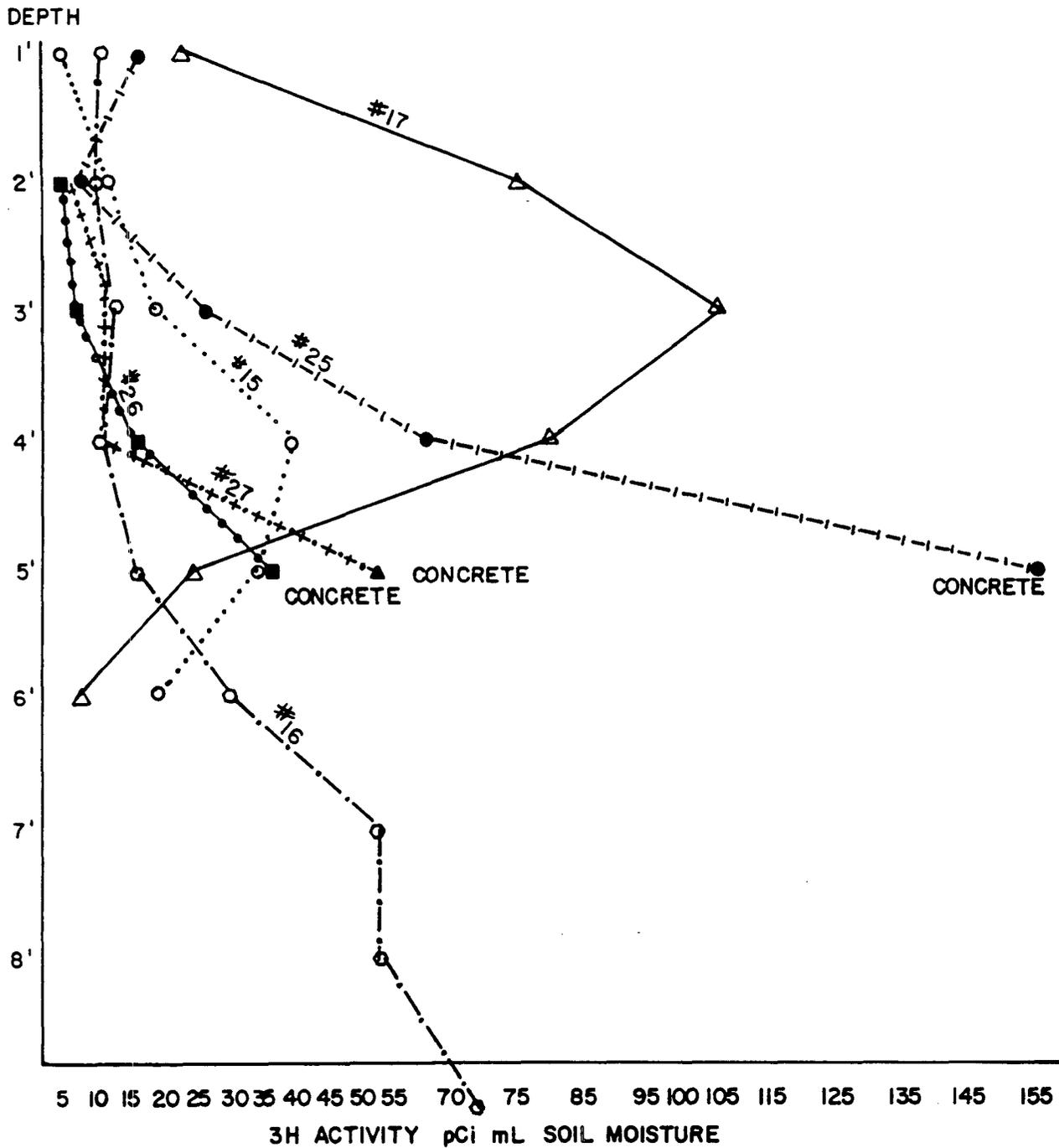
FIG.9 TRITIUM ACTIVITY VS DEPTH FOR PROFILE HOLES NORTH OF FLARE STACK
