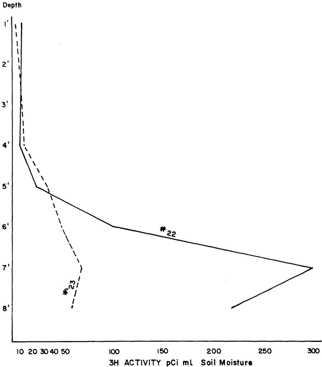
FIG.7 TRITIUM ACTIVITY VS DEPTH FOR PROFILE HOLES 22 EINI 10'N 18'W
