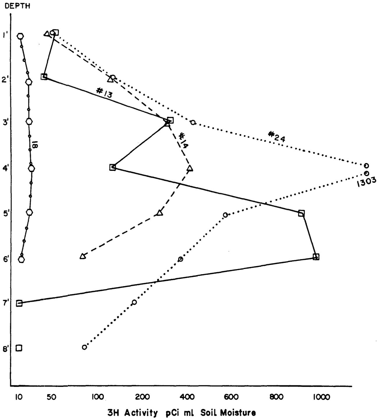
FIG.8 TRITIUM ACTIVITY VS DEPTH FOR PROFILE HOLES SOUTH OF FLARE STACK
