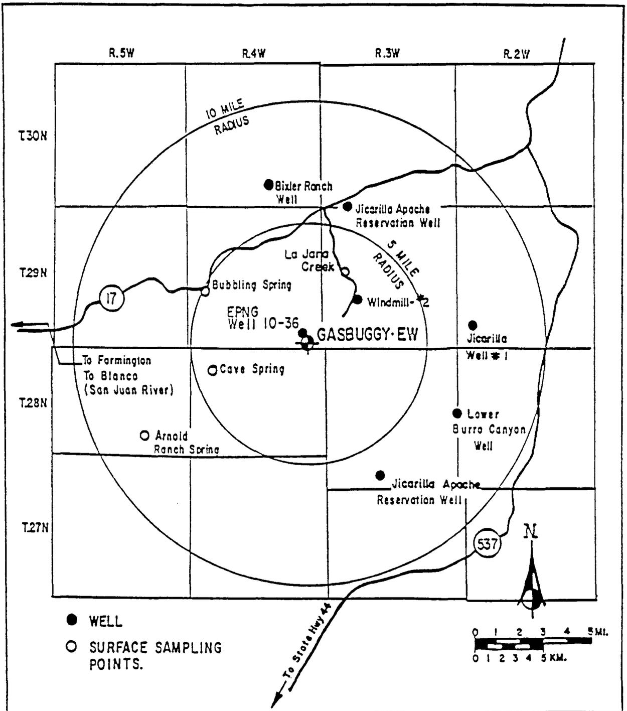
FIGURE 3.7.9. Long-Term Hydrologic Monitoring Program Sampling Points.
