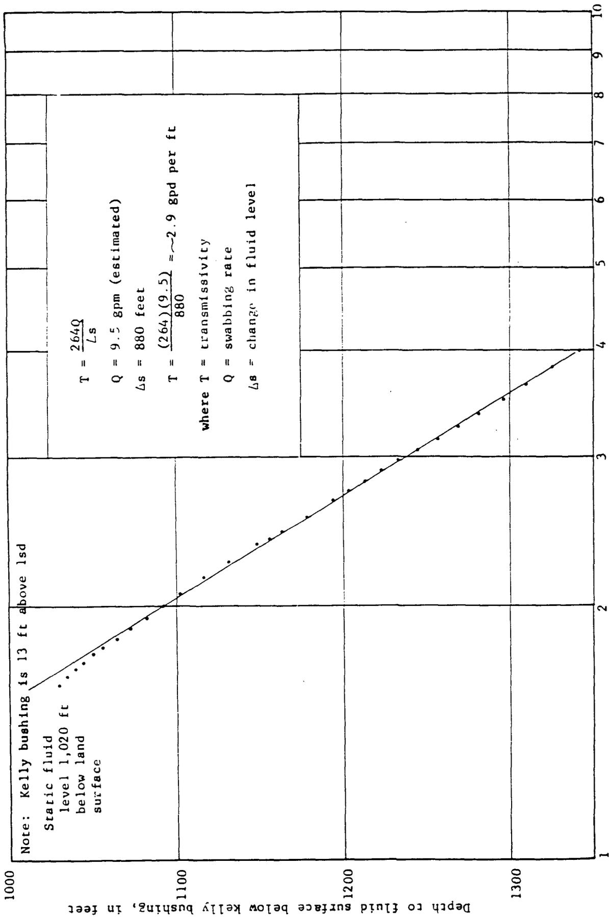
Figure 9.--Recovery of water level in hole GB-2 after swabbing test of Ojo Alamo Sandstone, April 17, 1967.
