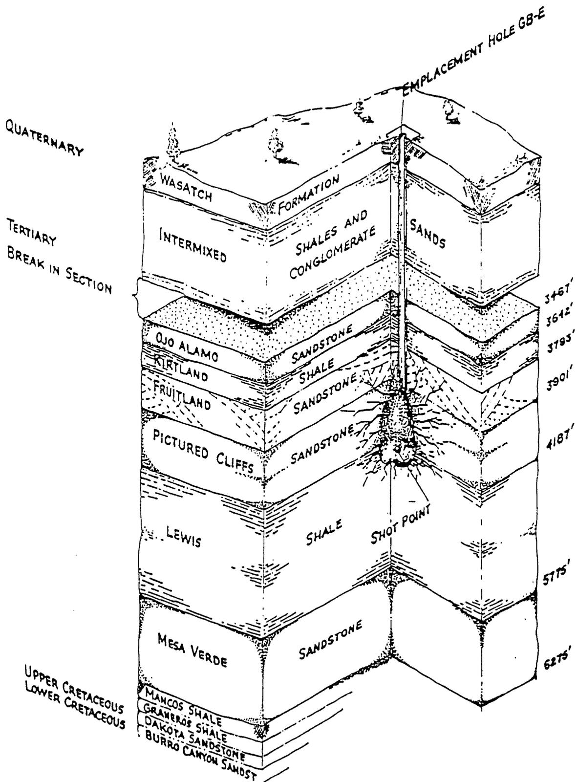
FIGURE 3.7.6. Project Gasbuggy Generalized Geologic Cross Section.
