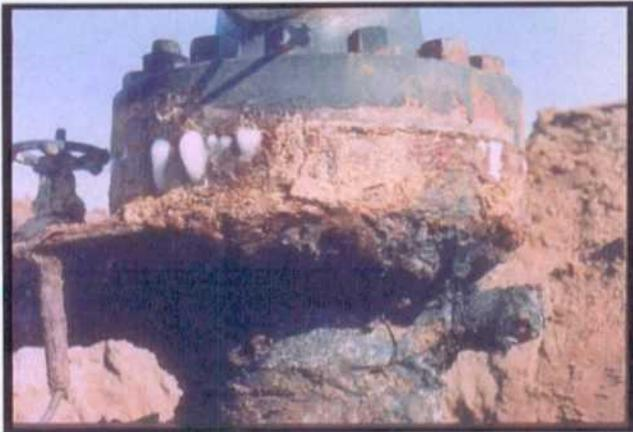
An example of a ring gasket failure at a CO<sub>2</sub> injection well in West Texas. The leak resulted in the formation of ice at the junction of two buried flange faces. Note the characteristic sulfide embrittlement on the surface of the casing head.
