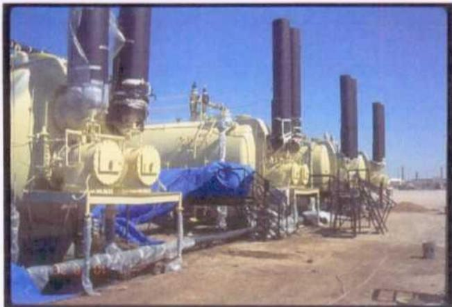
All surfaces are blasted to white metal, primed and painted with epoxy paint formulated to last for many years.
