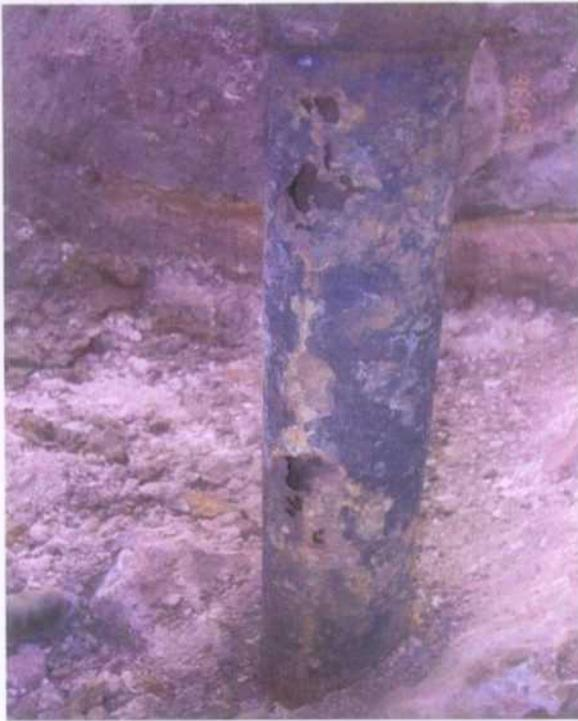
Example of corroded surface casing on a production well in South Texas. Ultrasonic measurement of the intermediate string indicated an 85% loss in thickness.
