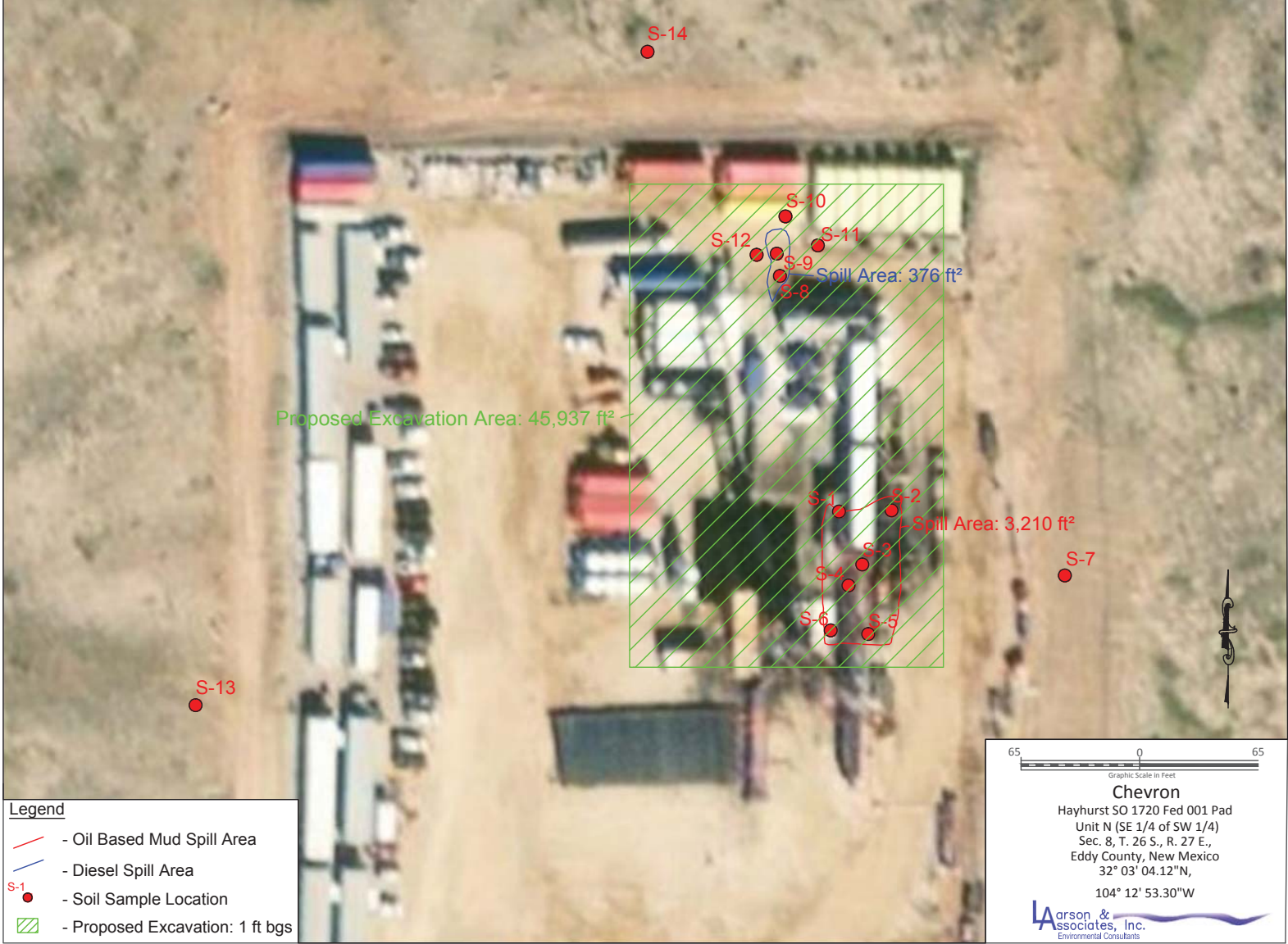
Figure 3 - Aerial Map Showing Proposed Excavation Location
