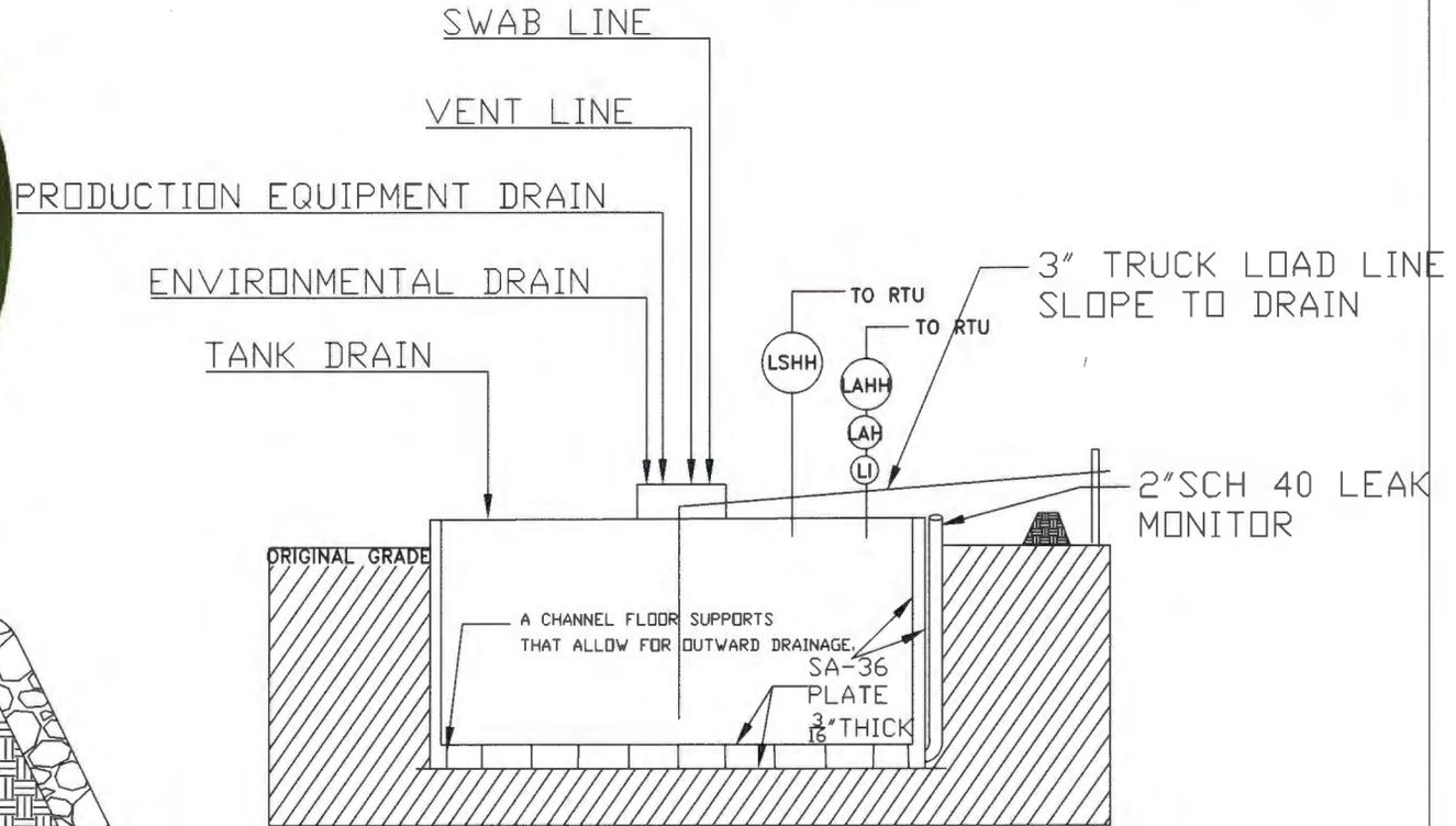
PROPERLY CONSTRUCTED FOUNDATION CONSISTING OF A LEVEL BASE FREE OF ROCKS, DEBRIS, SHARP EDGES OR IRREGULARITIES TO PREVENT PUNCTURES CRACKS OR INDENTATIONS TO THE TANK BOTTOM.
