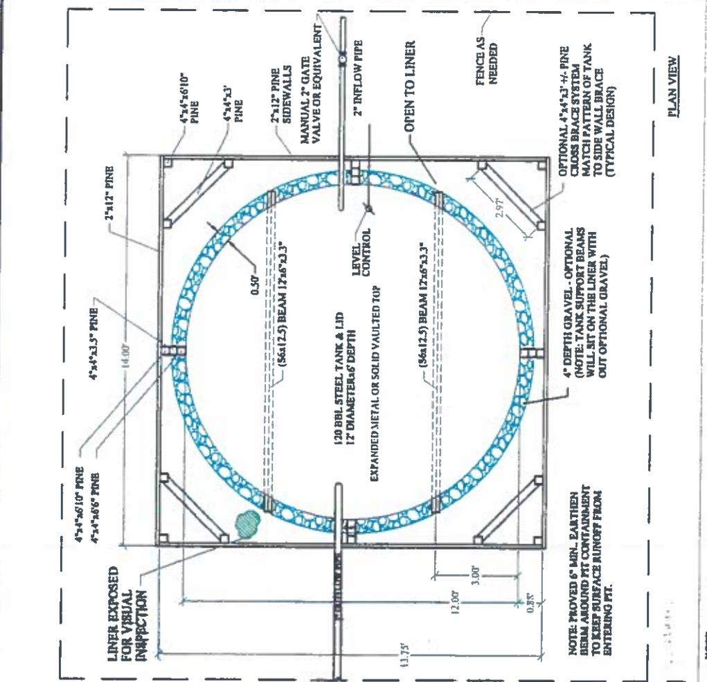
**NOTE: PROVIDED 6" MIN. EARTHEN BEAM AROUND FIT CONTAINMENT TO KEEP SURFACE RUNOFF FROM ENTERING FIT.**
