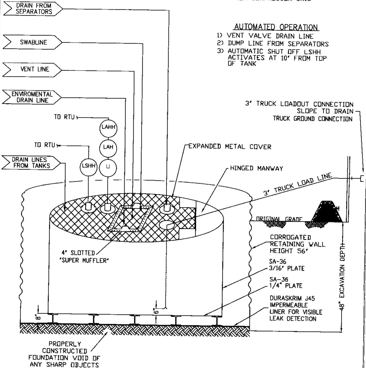
3" TRUCK LOADOUT CONNECTION
