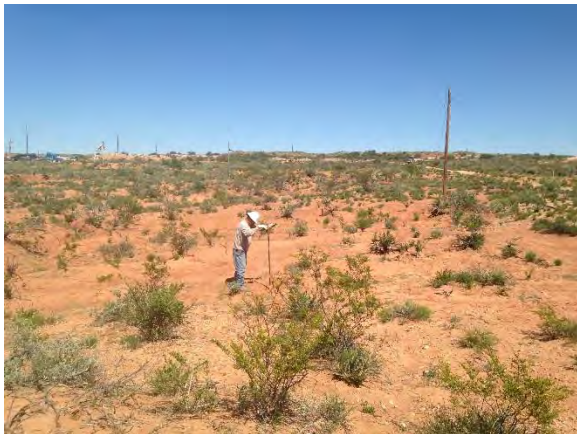
Collecting sample by hand auger, facing east
