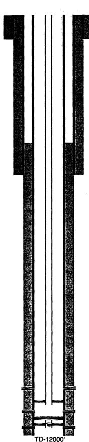
17-1/2" hole @ 650' 13-3/8" csg @ 650' w/ 715sx-TOC-Surf-Circ
