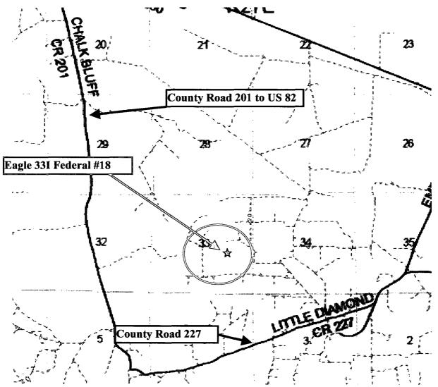
Assumed 100 ppm ROE = 3000° (Radius of Exposure) 100 ppm H2S concentration shall trigger activation of this plan.
