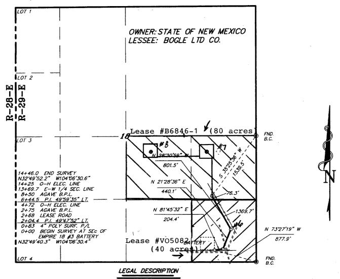
A STRIP OF LAND 30.0 FEET WIDE, LOCATED IN SECTION 18, TOWNSHIP 17 SOUTH, RANGE 29 EAST, N.M.P.M., EDDY COUNTY, NEW MEXICO AND BEING 15.0 FEET LEFT AND RIGHT OF THE FOLLOWING DESCRIBED CENTERLINE SURVEY.
