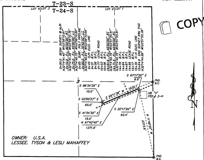
A STRIP OF LAND 30.0 FEET WIDE, LOCATED IN SECTION 3, TOWNSHIP 24 SOUTH, RANGE 29 EAST, N.M.P.M., EDDY COUNTY, NEW MEXICO AND BEING 15.0 FEET LEFT AND RIGHT OF THE ABOVE PLATTED CENTERLINE SURVEY.
