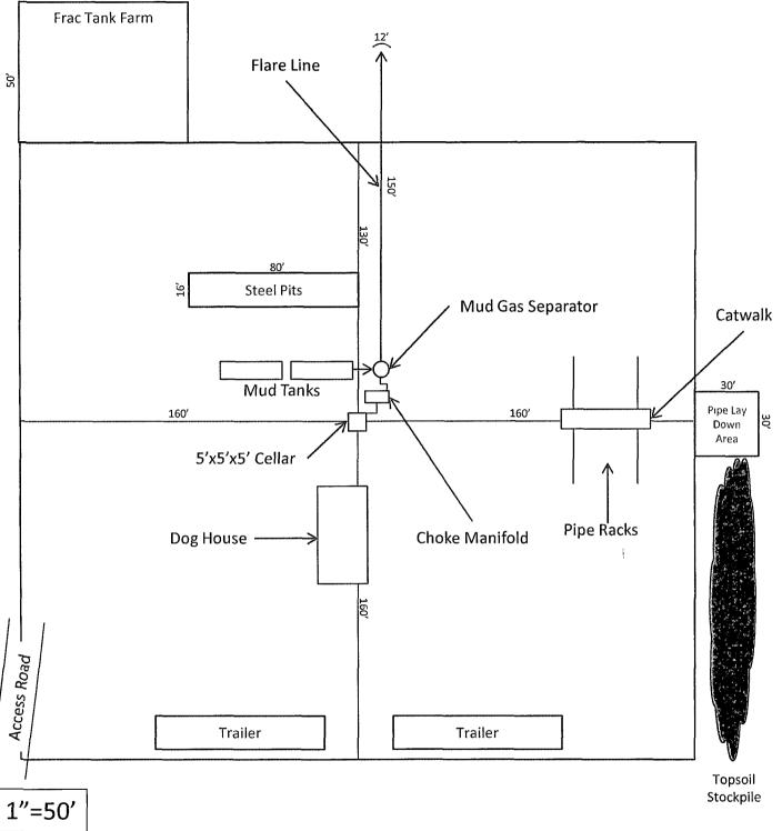
Exhibit D - Rig Diagram Sarvis 3 Federal Com No. 1 Cimarex Energy Co. of Colorado 3-26S-26E SHL 690 FNL & 400 FEL BHL 660 FNL & 660 FWL Eddy County, NM
