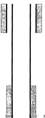
11" hole @ 724' 8-5/8" csg @ 724' w/ 250sx-TOC-Surf-Circ
