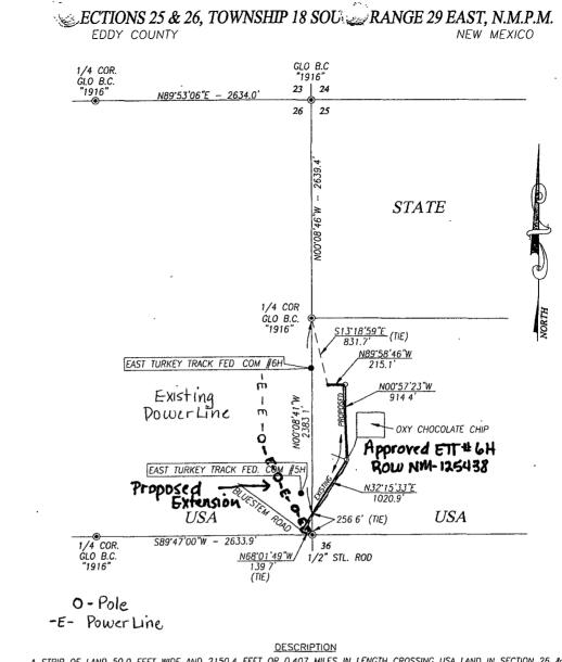
A STRIP OF LAND 50 O FEET WIDE AND 2150.4 FEET OR 0 407 MILES IN LENGTH CROSSING USA LAND IN SECTION 26 & 25. TOWNSHIP 18 SOUTH, RANGE 29 EAST, NMPM, EDDY COUNTY, NEW MEXICO AND BEING 25 O FEET LEFT AND 25 O FEET RIGHT OF THE ABOVE PLATTED CENTERLINE SURVEY
