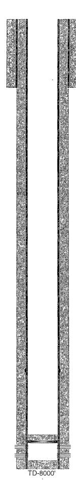
12-1/4" hole @ 1212' 9-5/8" csg @ 1212' w/ 600sx-TOC-Surf-Circ
