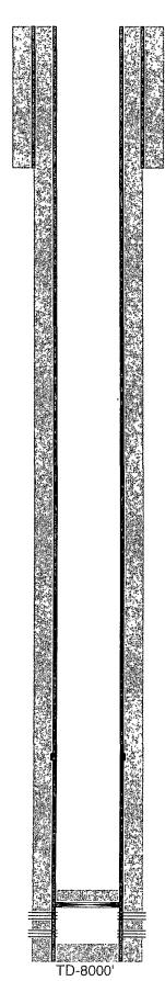
12-1/4" hole @ 1212' 9-5/8" csg @ 1212' w/ 600sx-TOC-Surf-Circ
