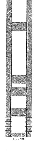
8-3/4" hole @ 8090' 7" csg @ 8090' DVT @ 6390' w/ 1035sx-TOC-Surf-Circ
