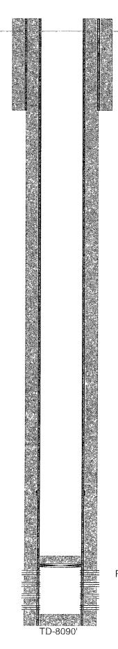
12-1/4" hole @ 1230' 9-5/8" csg @ 1230' w/ 800sx-TOC-Surf-Circ
