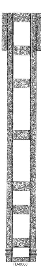
12-1/4" hole @ 1212' 9-5/8" csg @ 1212' w/ 600sx-TOC-Surf-Circ
