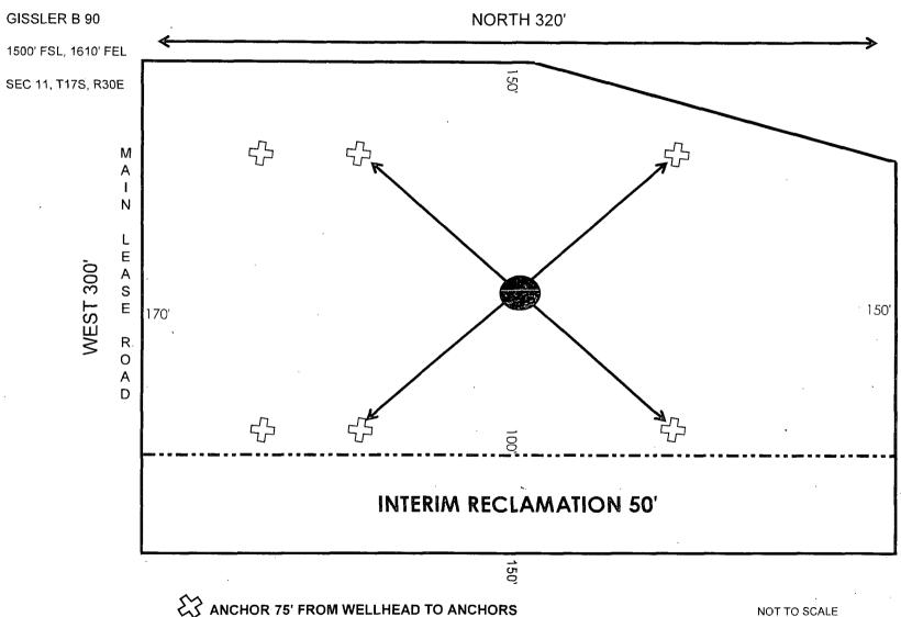
★ ANCHOR 75' FROM WELLHEAD TO ANCHORS **WELLHEAD**
