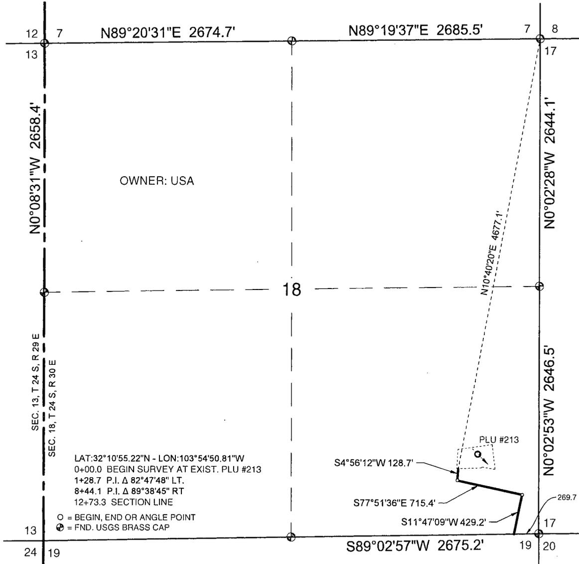
A STRIP OF LAND 30 FEET IN WIDTH, 1273.3 FEET, 0:24 MILE OR 77.2 RODS IN LENGTH, SITUATED IN SECTION 18, TOWNSHIP 24 SOUTH, RANGE 30 EAST, N.M.P.M., EDDY COUNTY, NEW MEXICO, AND BEING 15 FEET LEFT AND 15 FEET RIGHT OF THE SURVEY OF CENTERLINE AS SHOWN HEREON.
