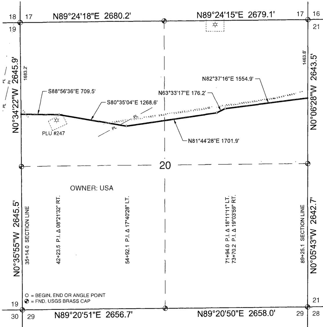
A STRIP OF LAND 30 FEET IN WIDTH, 5411.1 FEET, 1.02 MILES OR 327.95 RODS IN LENGTH, SITUATED IN SECTION 20, TOWNSHIP 24 SOUTH, RANGE 30 EAST, N.M.P.M., EDDY COUNTY, NEW MEXICO, AND BEING 15 FEET LEFT AND 15 FEET RIGHT OF THE SURVEY OF CENTERLINE AS SHOWN HEREON.
