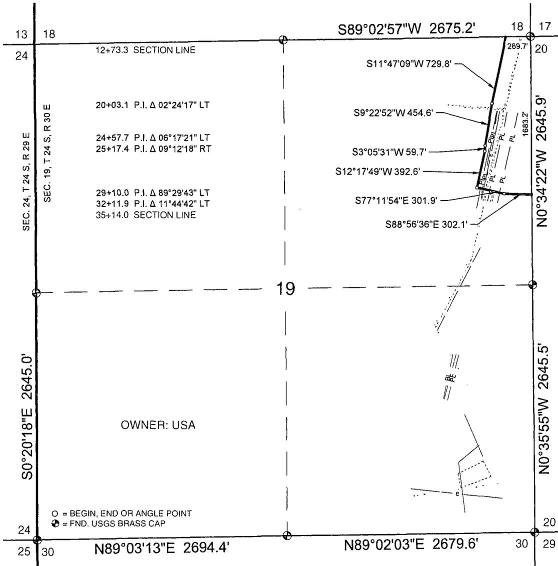
A STRIP OF LAND 30 FEET IN WIDTH, 2240.7 FEET, 0.42 MILE OR 135.80 RODS IN LENGTH, SITUATED IN SECTION 19, TOWNSHIP 24 SOUTH, RANGE 30 EAST, N.M.P.M., EDDY COUNTY, NEW MEXICO, AND BEING 15 FEET LEFT AND 15 FEET RIGHT OF THE SURVEY OF CENTERLINE AS SHOWN HEREON.
