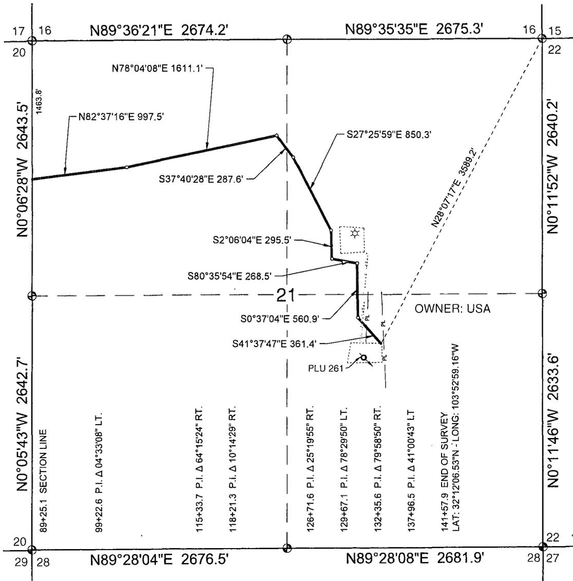
A STRIP OF LAND 30 FEET IN WIDTH, 5232.8 FEET, 0.99 MILE OR 317.1 RODS IN LENGTH, SITUATED IN SECTION 21, TOWNSHIP 24 SOUTH, RANGE 30 EAST, N.M.P.M., EDDY COUNTY, NEW MEXICO, AND BEING 15 FEET LEFT AND 15 FEET RIGHT OF THE SURVEY OF CENTERLINE AS SHOWN HEREON.
