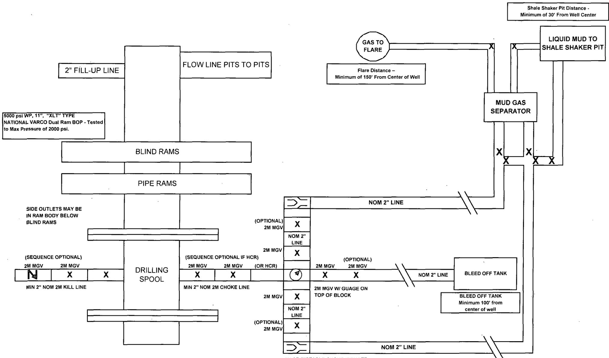
2M ADJUSTABLE CHOKE (REMOTE OPERATED CHOKE OPTIONAL FOR ONE SIDE ONLY)
