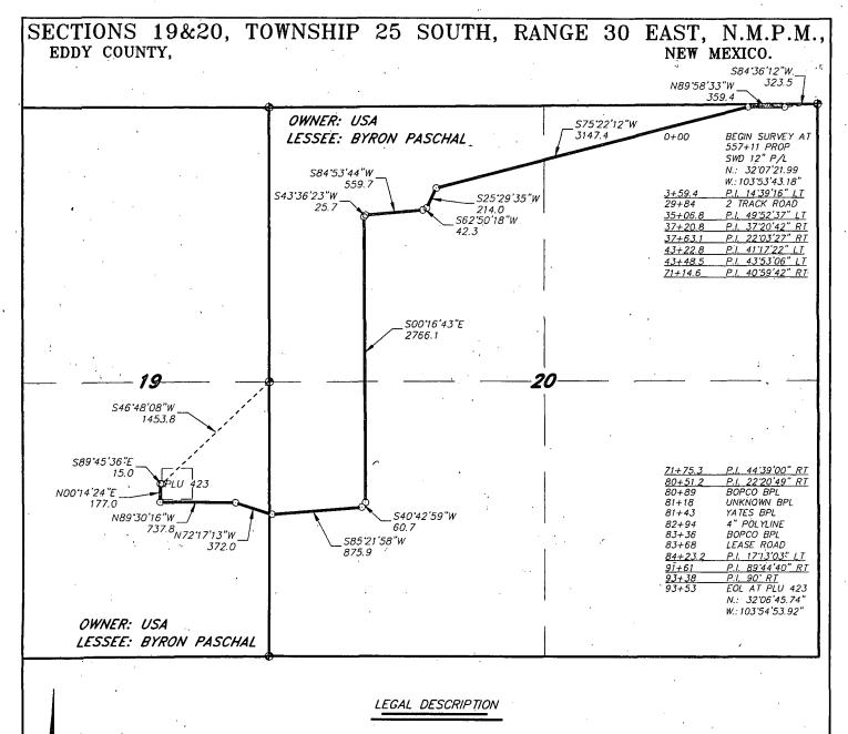
A STRIP OF LAND 30.0 FEET WIDE, LOCATED IN SECTIONS 19&20, TOWNSHIP 25 SOUTH, RANGE 30 EAST, N.M.P.M., EDDY COUNTY, NEW MEXICO AND BEING 15.0 FEET LEFT AND RIGHT OF THE ABOVE PLATTED CENTERLINE SURVEY.
