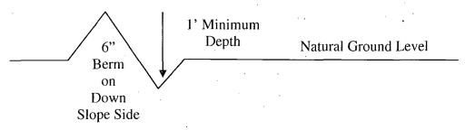
All lead-off ditches shall be graded to drain water with a 1 percent minimum to 3 percent maximum ditch slope. The spacing interval are variable for lead-off ditches and shall be determined according to the formula for spacing intervals of lead-off ditches, but may be amended depending upon existing soil types and centerline road slope (in %);
