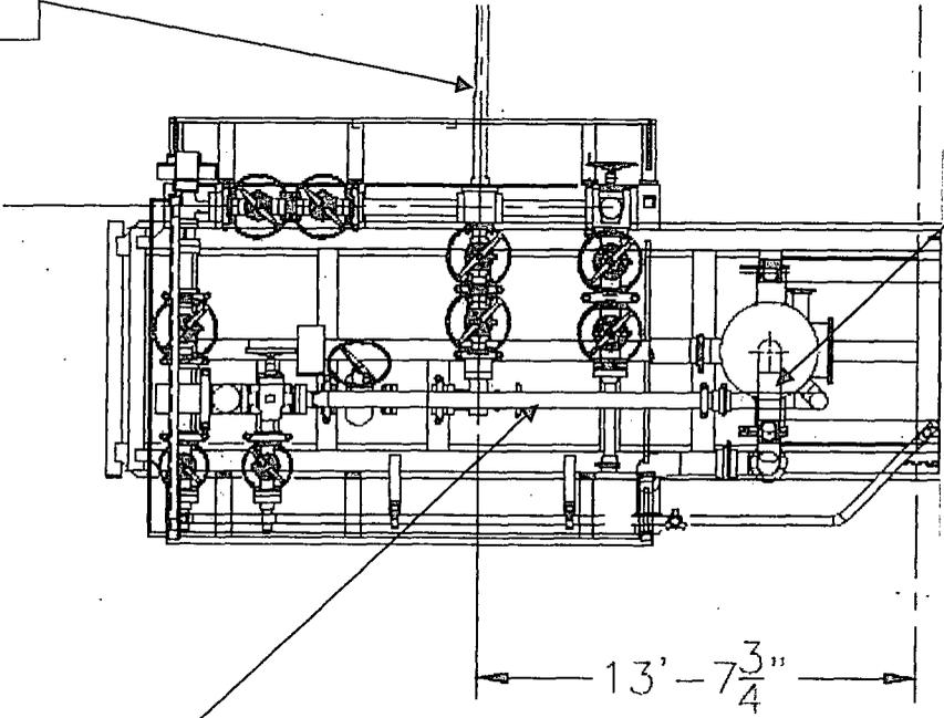
**Choke Manifold - Gas Separator (Side View)**
