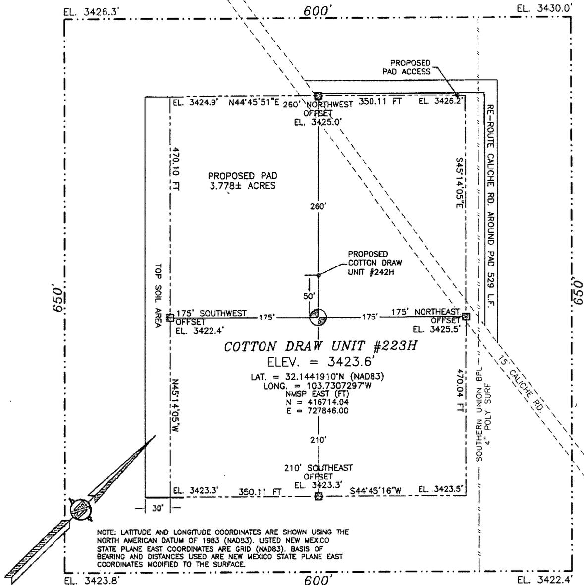
NOTE: LATITUDE AND LONGITUDE COORDINATES ARE SHOWN USING THE NORTH AMERICAN DATUM OF 1983 (NAD83). LISTED NEW MEXICO STATE PLANE EAST COORDINATES ARE GRID (NAD83). BASIS OF BEARING AND DISTANCES USED ARE NEW MEXICO STATE PLANE EAST COORDINATES MODIFIED TO THE SURFACE.
