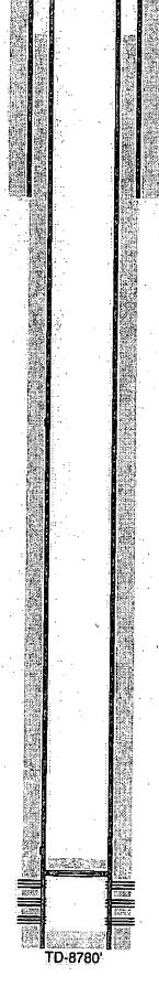
12-1/4" hole @ 1825' 9-5/8" csg @ 1820' w/ 993sx-TOC-Surf-Circ
