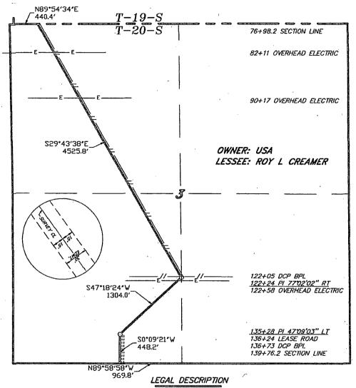
A STRIP OF LAND 30.0 FEET WIDE, LOCATED IN SECTION 3, TOWNSHIP 20 SOUTH, RANGE 31 EAST, N.M.P.M., EDDY COUNTY, NEW MEXICO AND BEING 15.0 FEET LEFT AND RIGHT OF THE ABOVE PLATTED CENTERLINE SURVEY.
