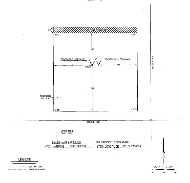
ALL BEARINGS, DISTANCES, AND COORDINATE VALUES CONTAINED HEREON ARE GRID BASED UPON THE NEW MEXICO STATE PLANE COORDINATE SYSTEM, EAST ZONE OF THE NORTH AMERICAN DATUM 1927, U.S. SURVEY FEET
