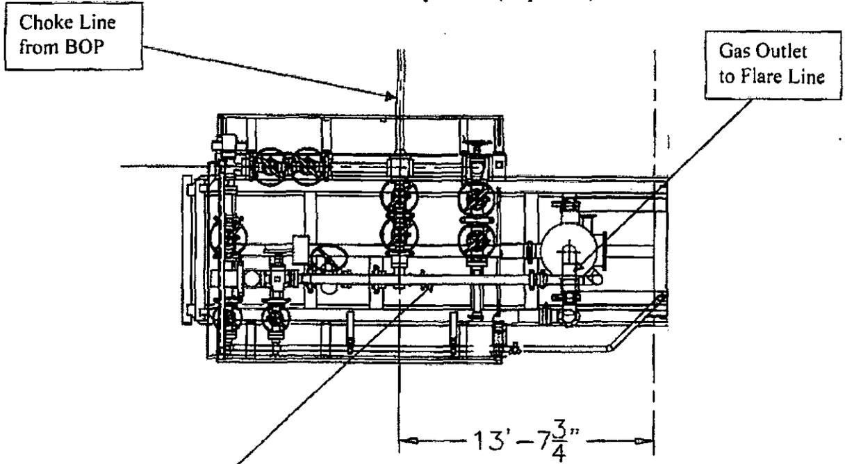
Choke Manifold - Gas Separator (Side View)
