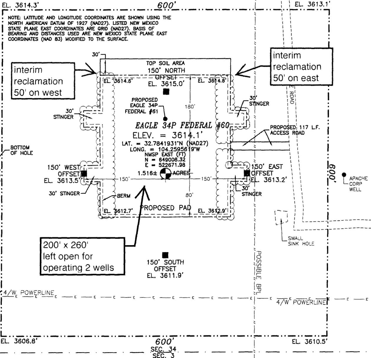
NOTE: LATITUDE AND LONGITUDE COORDINATES ARE SHOWN USING THE NORTH AMERICAN DATUM OF 1927 (NAD27). LISTED NEW MEXICO STATE PLANE EAST COORDINATES ARE GRID (NAD27). BASIS OF BEARING AND DISTANCES USED ARE NEW MEXICO STATE PLANE EAST COORDINATES (NAD 83) MODIFIED TO THE SURFACE.
