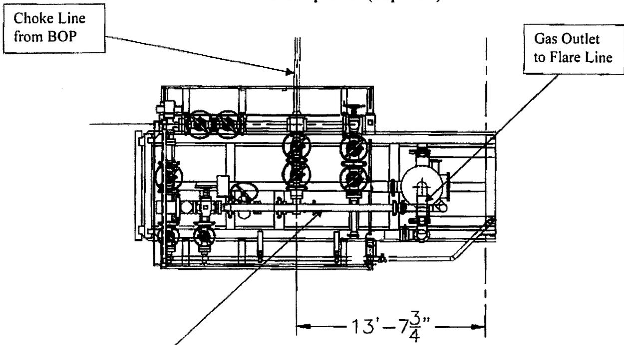
Choke Manifold – Gas Separator (Side View)
