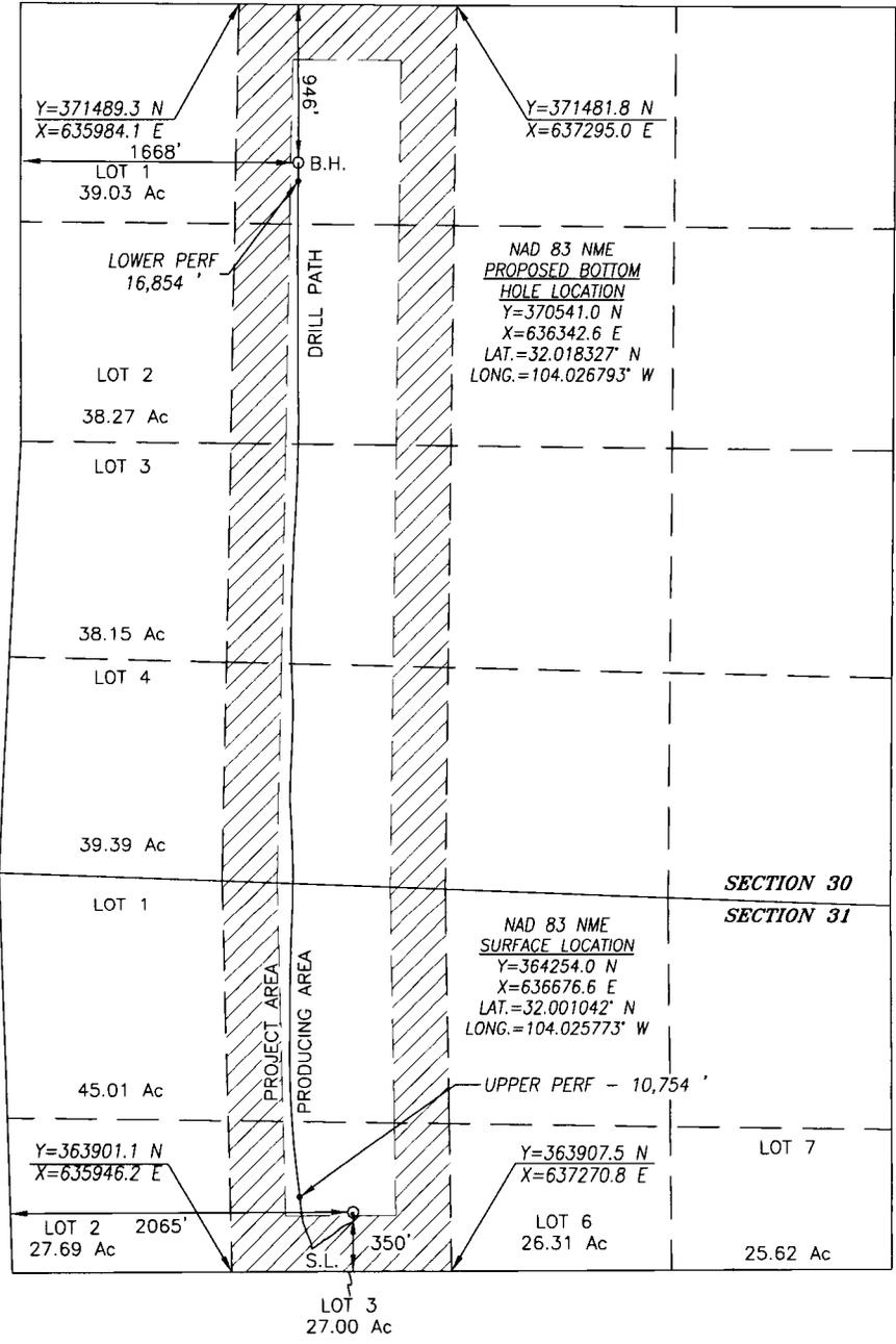
BOREPATH SHOWN HEREON IS BASED ON DIRECTIONAL SURVEY REPORT PROVIDED BY COG OPERATING, LLC FOR THE COPPERHEAD FEE A SUPPLIED TO HARCROW SURVEYING, LLC ON JULY 3, 2017.
